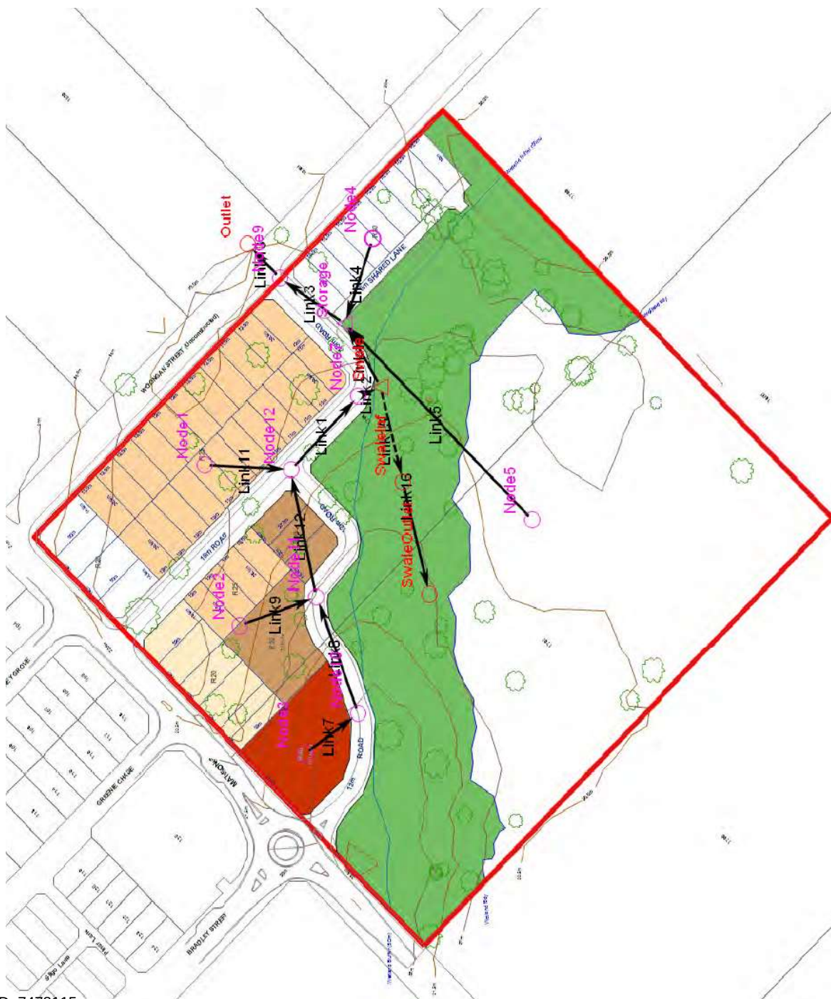
Figure 20: XP-Storm node delineation
